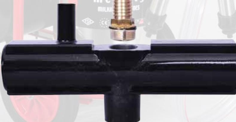
Due to vacuum tank outlet is smaller and air partition was made in narrow diameters, decrease in volumetric flow rate was discovered as a result of R & D carried out by Melasty. This problem was reduced with development of **Melasty 7005 Vacuum Distributor** with Inlet Ø30mm – outlet Ø24, 5mm and air tank vacuum outlet was upgraded to Ø32mm, thus makes machine breathes more comfortable.
